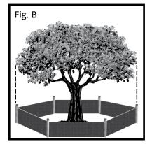
2. **Natural Areas** – To restrict access into areas where land alteration and construction activities are not authorized a physical structure not less than 3 feet in height is placed along the perimeter of such areas.
