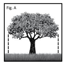
1. Trees – To restrict access into the area within the canopy dripline of a tree, a physical structure not less than 3 feet in height, comprised of wood or other suitable material, is placed around the tree at the canopy dripline, except where land alteration or construction activities are approved within the canopy dripline. The canopy dripline of a tree is the imaginary, vertical line that extends downward from the outermost tips of the tree's branches to the ground, as shown in Figure A.
